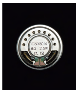
Icom custom high power handling capacity speaker
